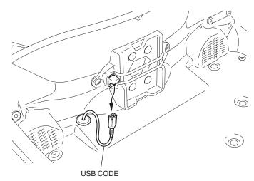
3. Remove the trunk holder as shown.Perform this step on GL1800DA only.
